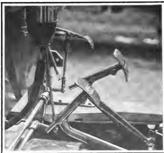
White foot pedals showing the means of adjustment whereby the operator is enabled to lengthen the pedal stems to suit his own individual requirements; also the accelerator pedal and the connections of the Bosch dual ignition system
